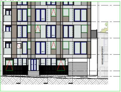
Referring to the acoustic report provided with the application by Earcon dated 16/12/2020, Section 4.5 regarding external doors with glazing refers to Section 4.3, where MetroGlass Laminate IGU (6.38 mm / 12mm AS / 6mm) is proposed.
